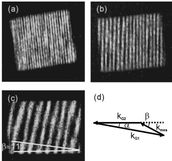
Fig. 3. Contrast-enhanced Moiré fringes recorded by a CCD camera through an optical microscope under  $p$ -polarized 376 nm illumination. The sample configurations are exactly the same as Fig. 2(c) except that the first chromium grating period is 120 nm in (a), 130 nm in (b), and 140 nm in (c). (d) Vector representation of the Moiré effect obtained by superposing two periodic gratings.
